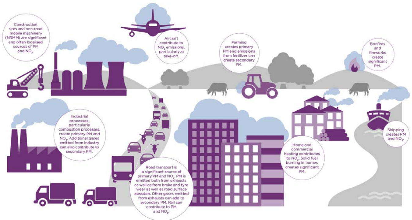
Figure 2: Sources of air pollution including oxides of nitrogen (NO x ) and fine particulate matter (PM 2.5 ) 6
